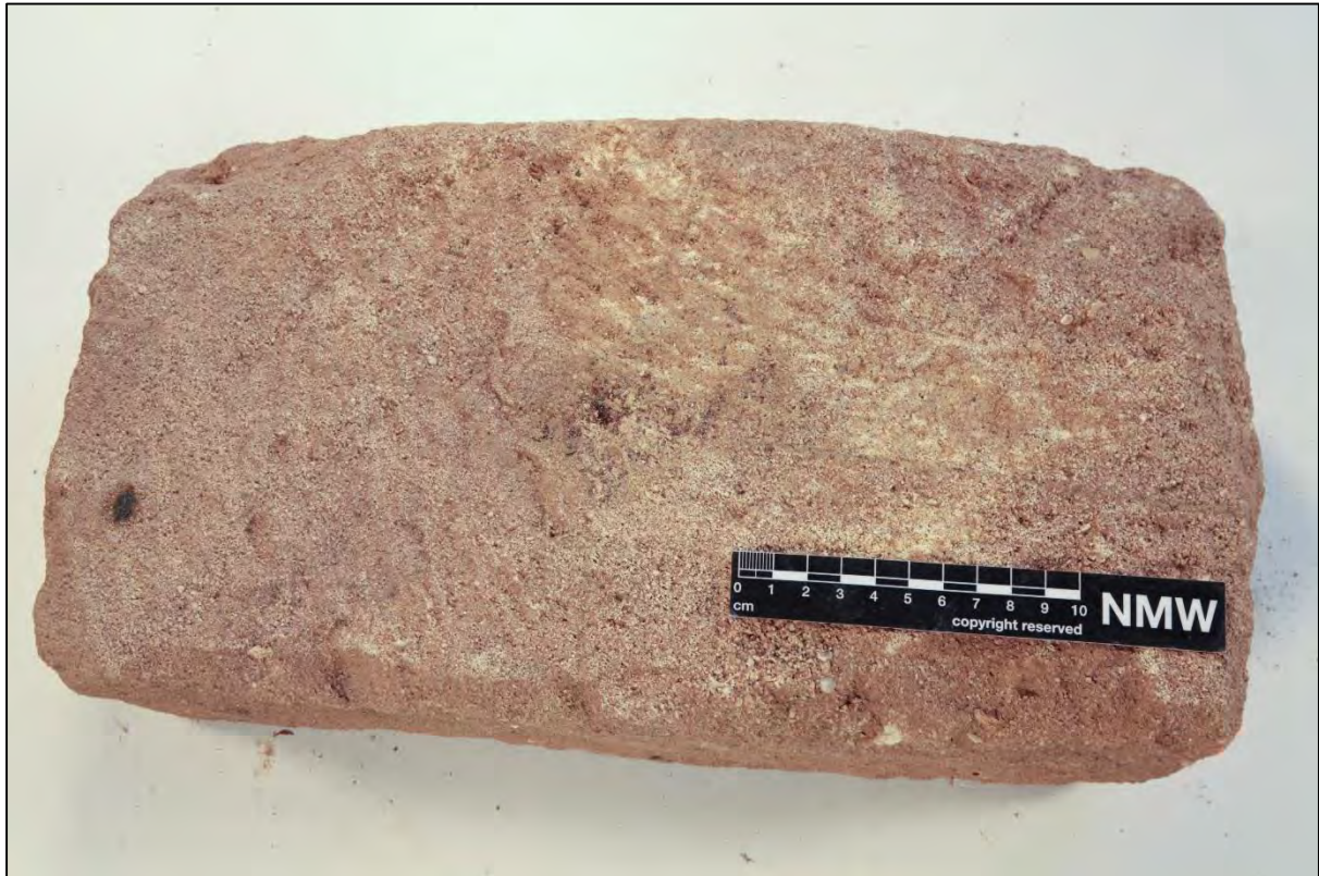
Figure 9: Specimen 24_8 - 8 of 9: Obvious masonry marks observed on large face of block (nearest viewer)
