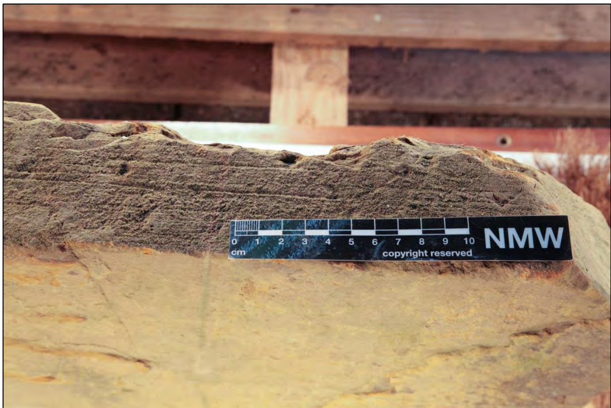
Figure 10: Specimen 71_25 1 of 3: Laminations observed in lateral face of block
