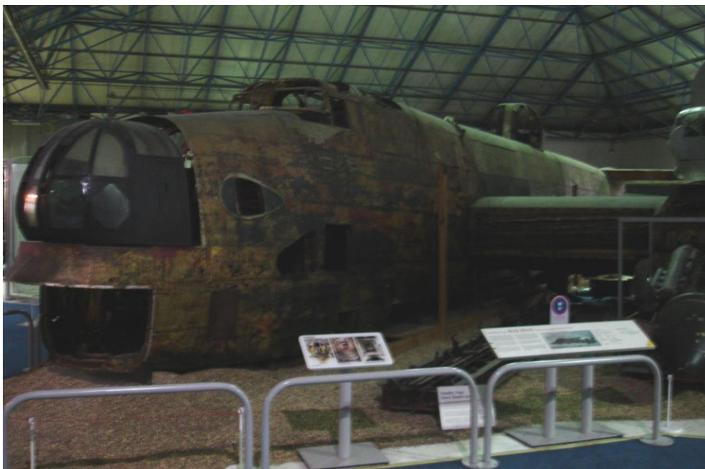
Figure 10 Halifax W1048 on display at RAFM London. Elements of the aircraft have been rebuilt, including the front gun turret. Image taken by the author.
