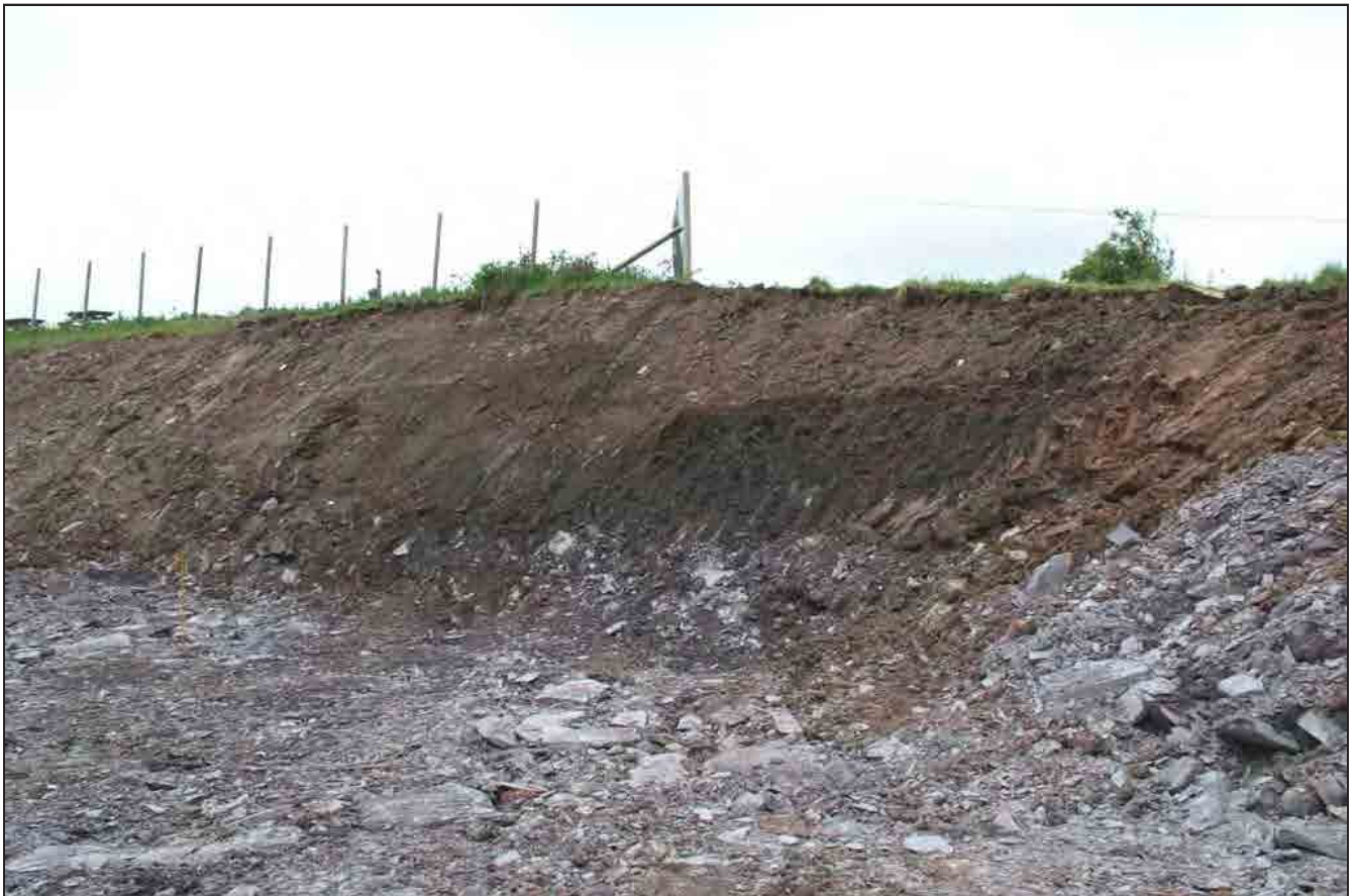
Plate 10: Exposed section showing made-ground deposits to the east of the site entrance. View from the west.
