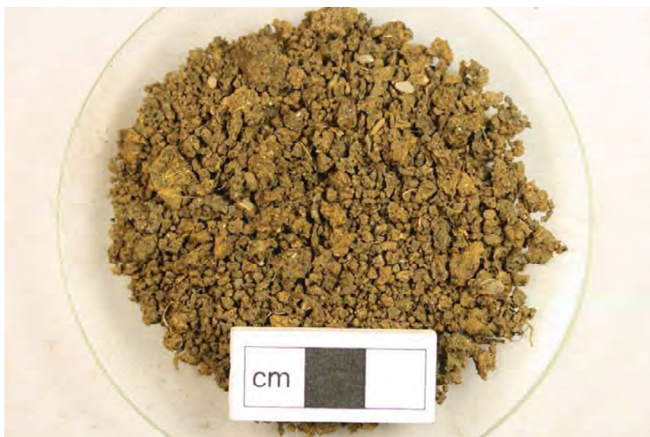
Plate 1: granular magnetic residue, probably roasted bog ore particles.
