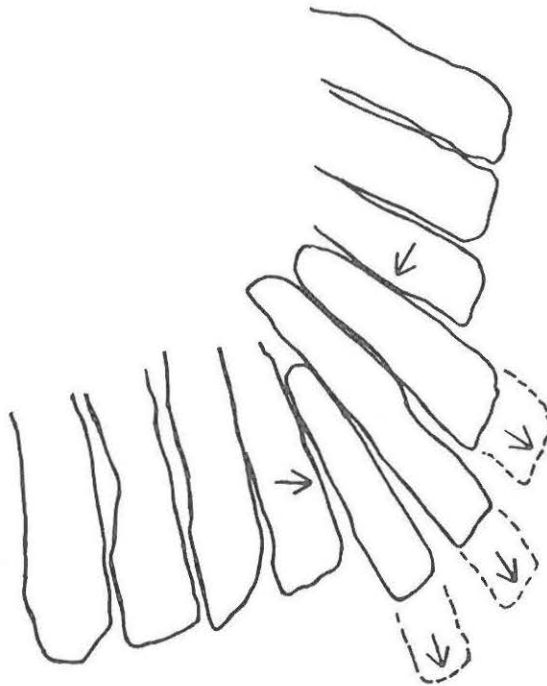
Fig. 4 Sketch plan illustrating the forces acting on stones in convex masonry
