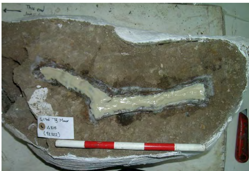
Figure 6: The epoxy resin support.
