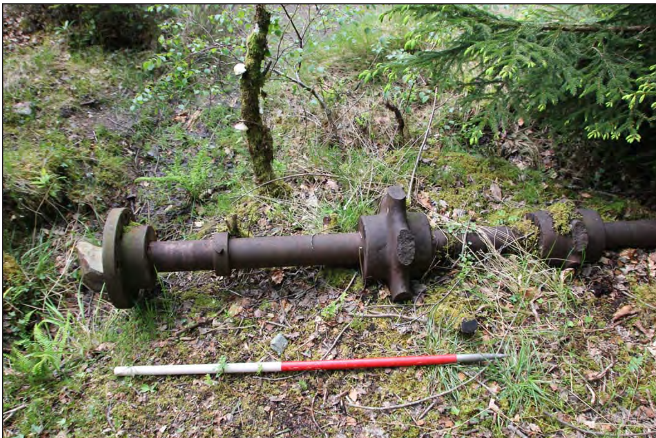
Plate 25: Mill central floor feature 8 showing stamp battery shaft, from the north. Scale 1.0m.
