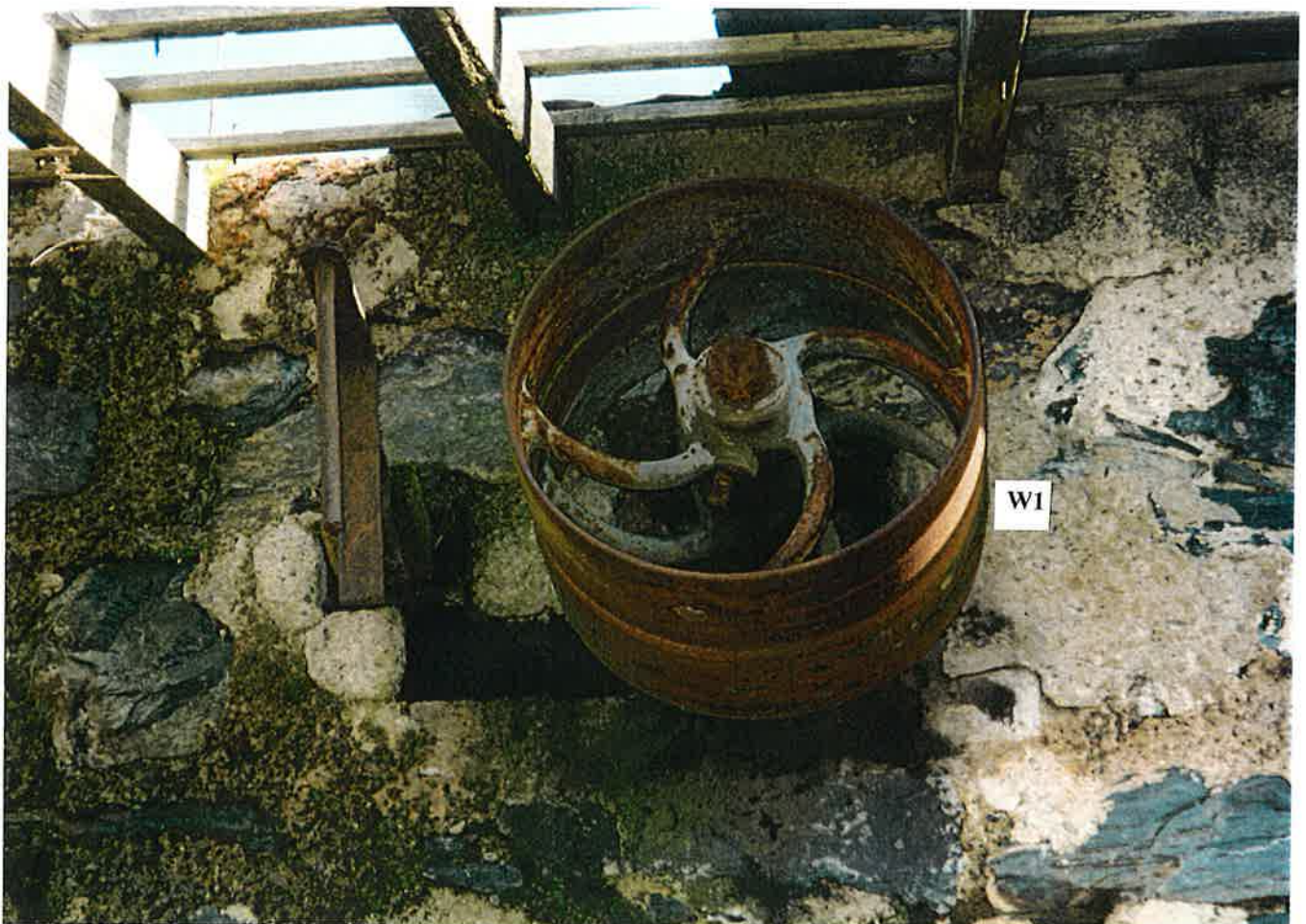
Plate 13 below: The cast iron 16" diameter belt drive wheel located on the outside wall of the barn, inside the lean-to engine compartment.
