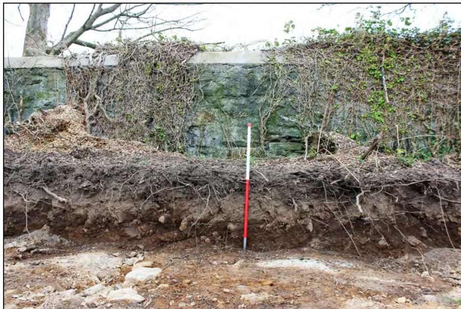
Plate 38: Sample section adjacent to east boundary showing depth of topsoil & subsoil natural stoney clay (garden area of Plot 121) May 2017
