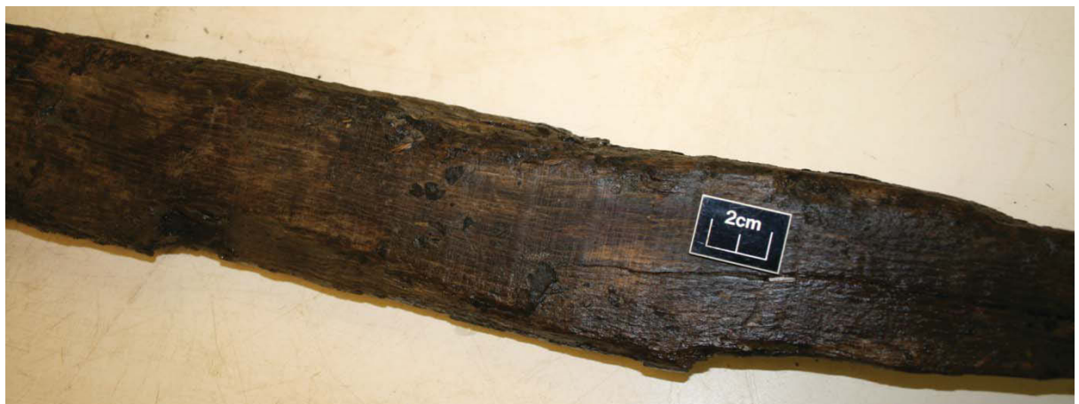
Figure 12.59 photograph of vertical saw marks(left of scale) on upper face of sample 52 4 of 4
