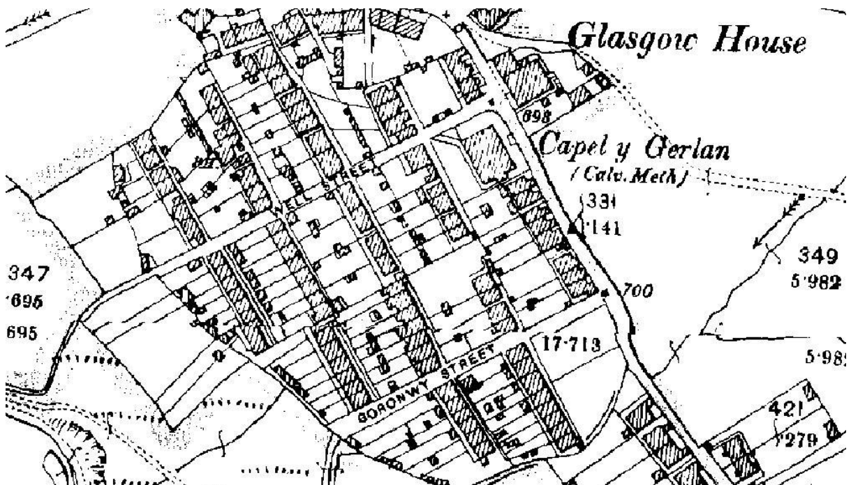
Fig 15 Gerlan in 1889. Houses are reached by communal paths and back courts at right angles to Well Street and Goronwy Street. The gardens are at the front, on the downhill (left in the picture) side of the houses.
