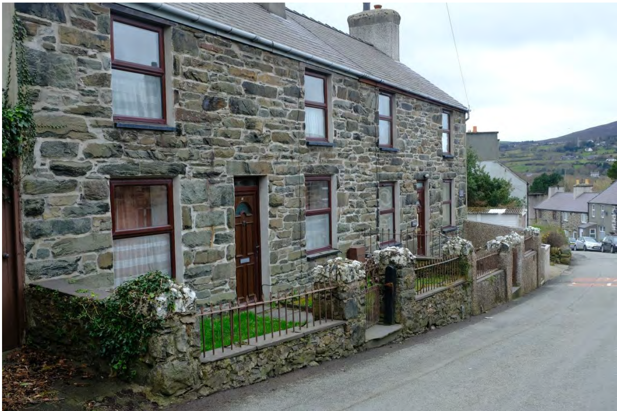
Fig 21 Most of Bethesda's houses, like this pair on Penybryn Road are built of quarried stone laid in rough courses. The copings of the gate piers are of small pieces of quartz, which was a by-product of slate quarrying.
