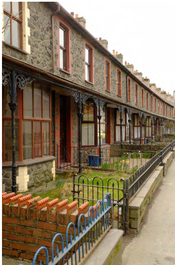
Fig 40 Gordon Terrace / Rhes Gordon, dated 1885, is a superior row of houses notable for the use of broken pieces of stone laid in a crazed pattern, and for the continuous veranda on cast-iron posts, a self-consciously non-local design.
