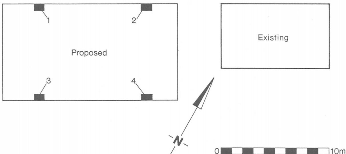
Fig. 2 Building footprint showing position of test pits
