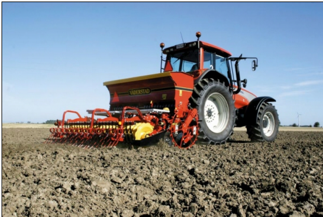
Fig. 16 An example of non-inversion tillage using the Väderstad Carrier Drill 300 (photo Väderstad)
