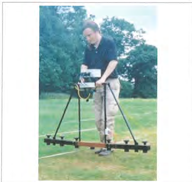
Figure 8 RM15 electrical resistance meter
