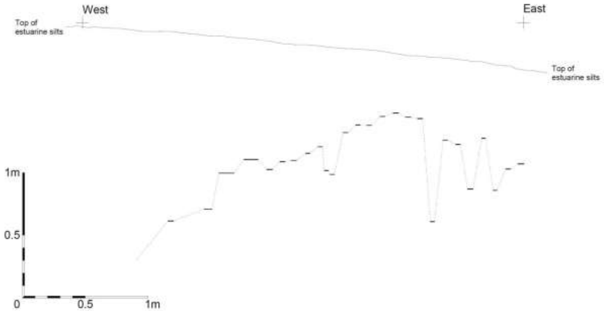
Figure 7: Profile 2 along the width of Wreck 2 (northern profile), with readings taken every 10cm. Depths shown are to the top of solid timbers (no timbers recorded to southwest)
