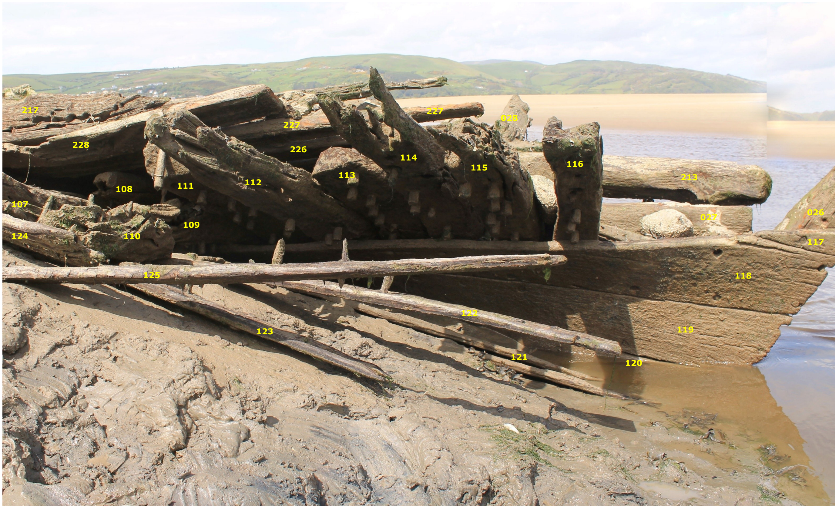
Photo 15: Port side of wreck showing frames and outer planking towards the stern (merged photographs from June 2015)
