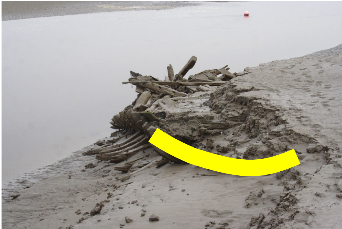
Photo 8: Bow end of the starboard side, with cant frames highlighted curving in towards bow stempost as revealed in 2014 excavation (March 2016)
