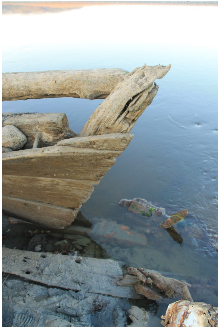
Photo 17: Stern of vessel on port side, showing lower timber projecting below the waterline with hole within it (September 2015)
