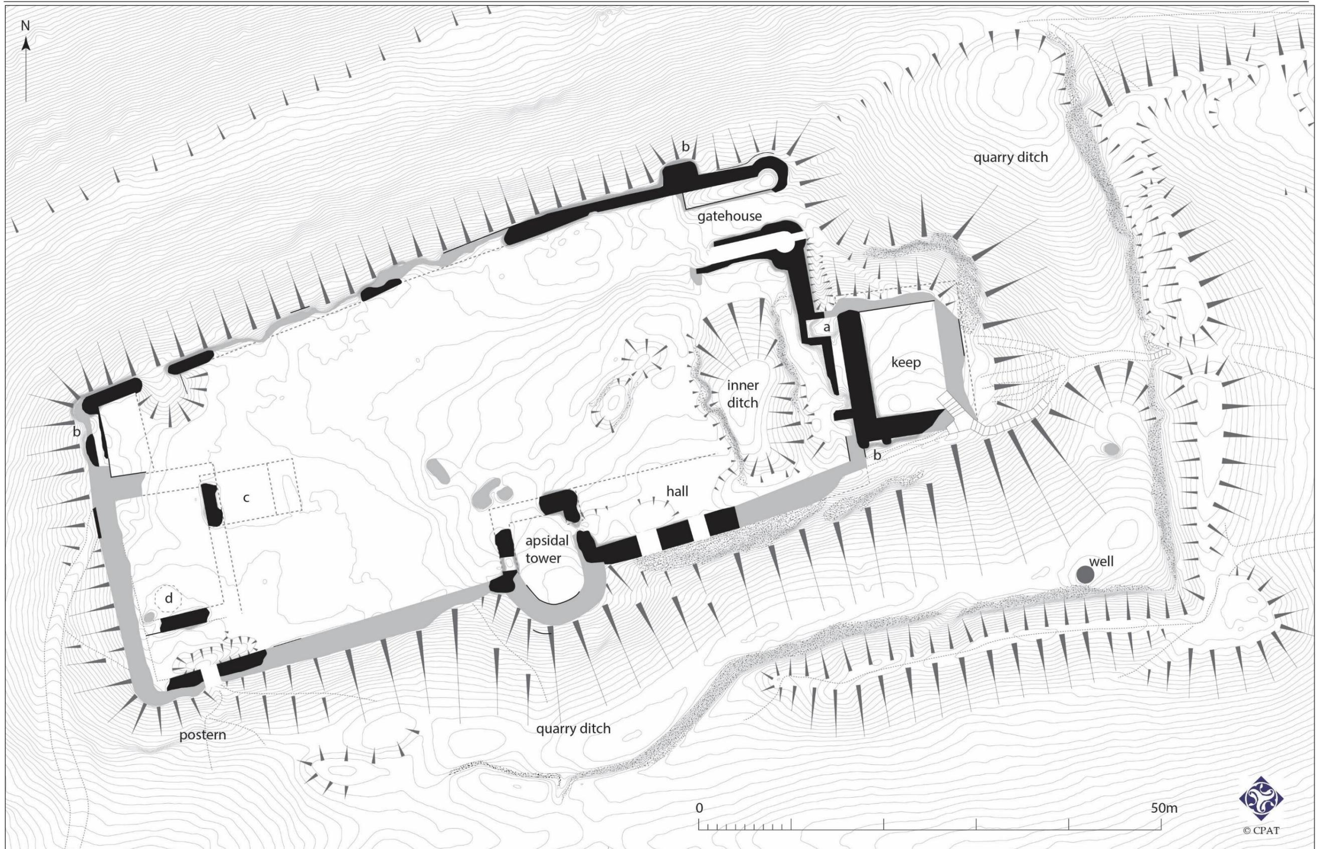
Fig. 7 Plan showing the masonry castle, with contours derived from the drone survey, courtesy of Mark Walters. a – stair access to keep, b – latrines, c – site of cottage, d – site of camera obscura
