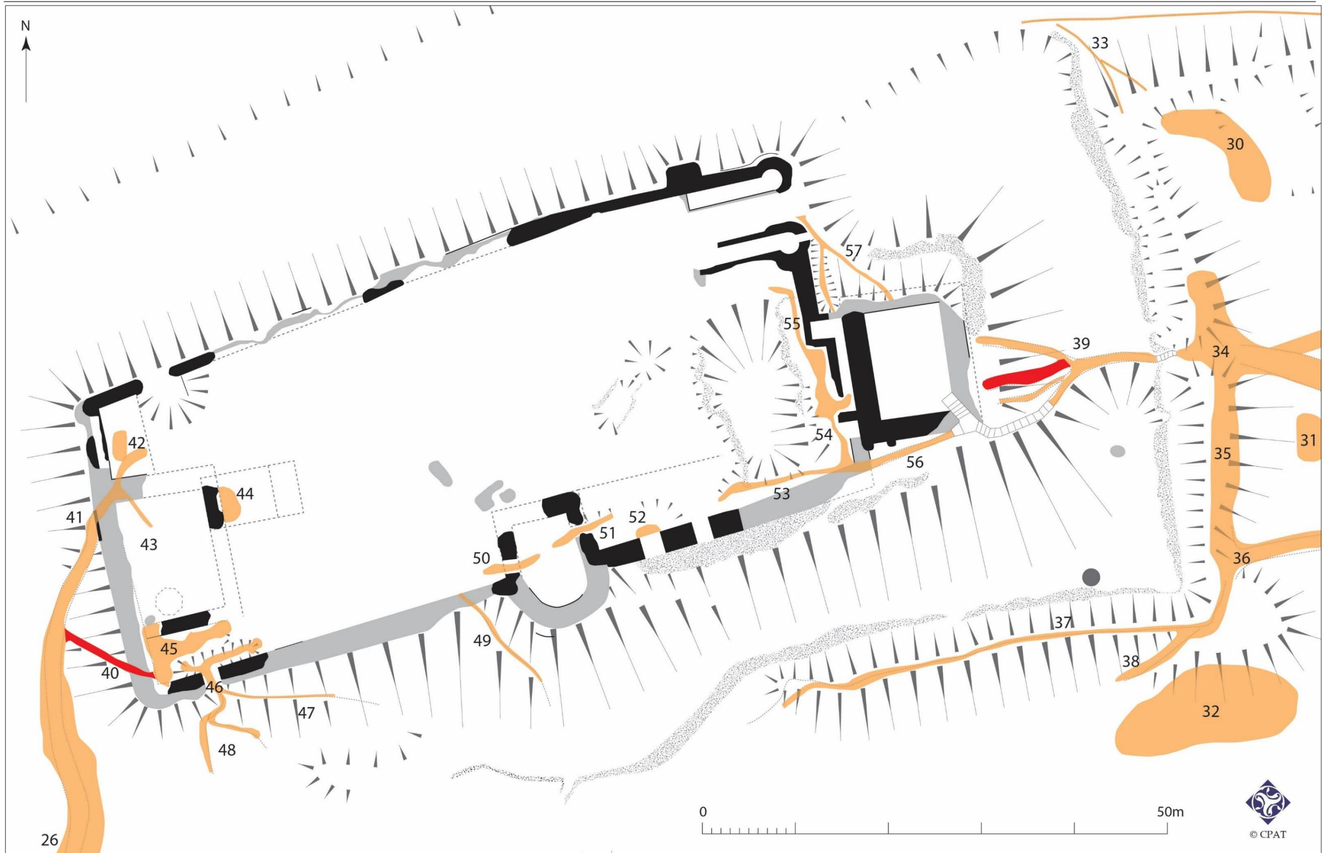
Fig. 10 Plan showing management issues within the masonry castle. Issues in red require remedial action.
