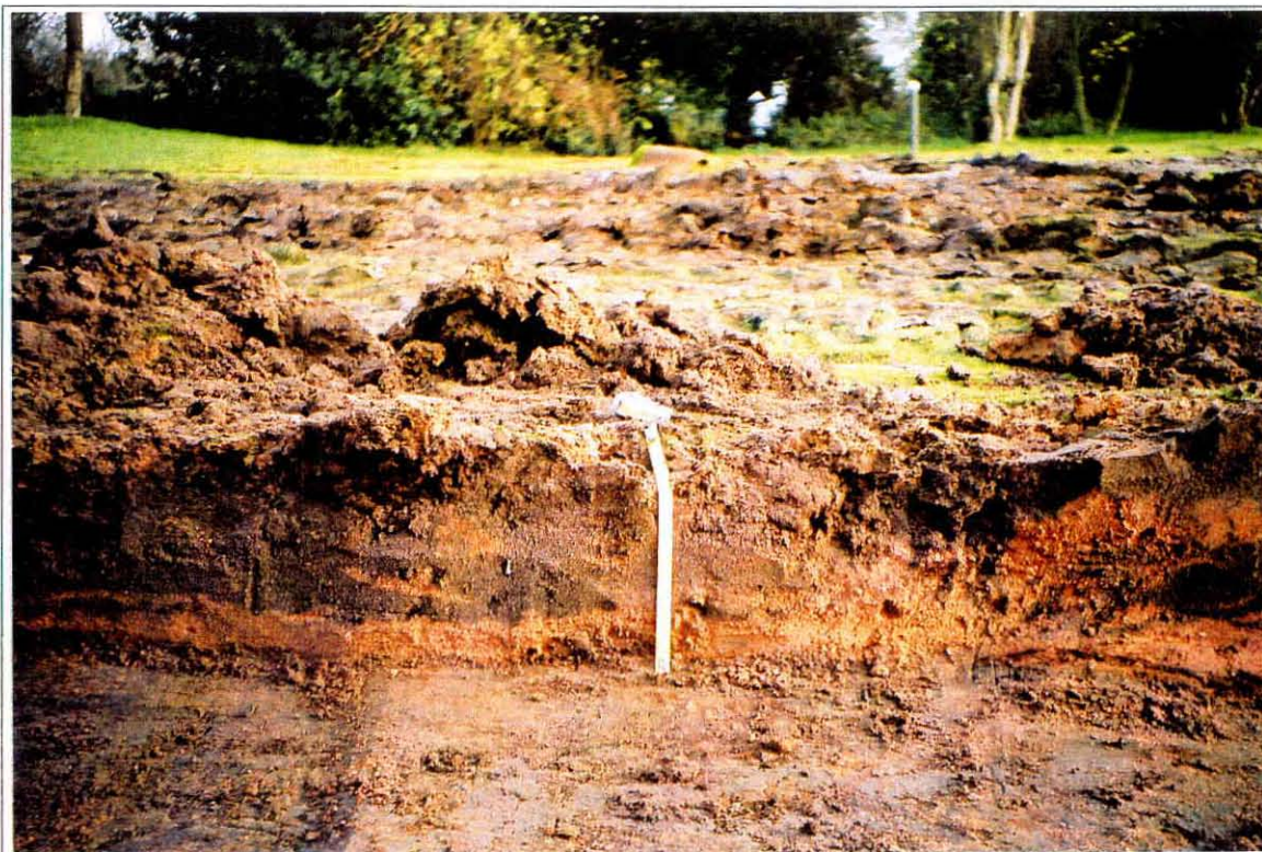
Plate 4 4th Green showing sand and peat make-up. Photo CPAT 1131.16
