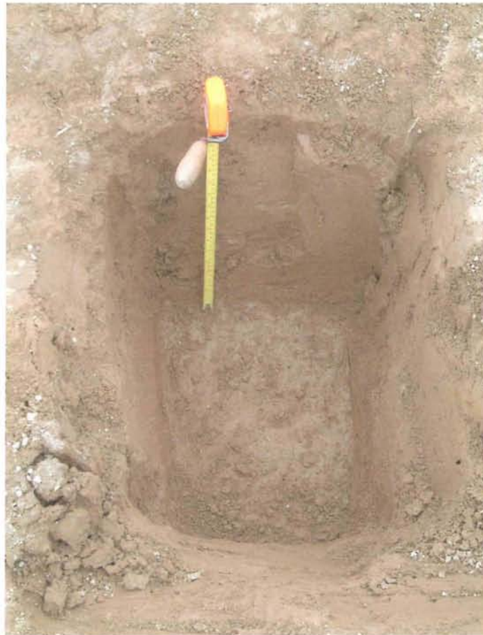
Plate 2: Example of 0.5m by 0.5m by 1m test pit dug to test the depth of the alluvial deposits.
