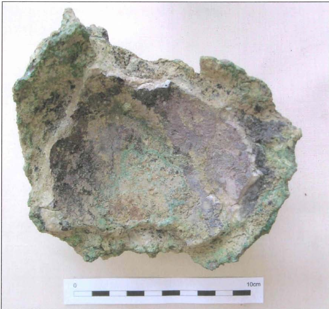
Plate 11 Copper alloy smelting hearth base from context 22
