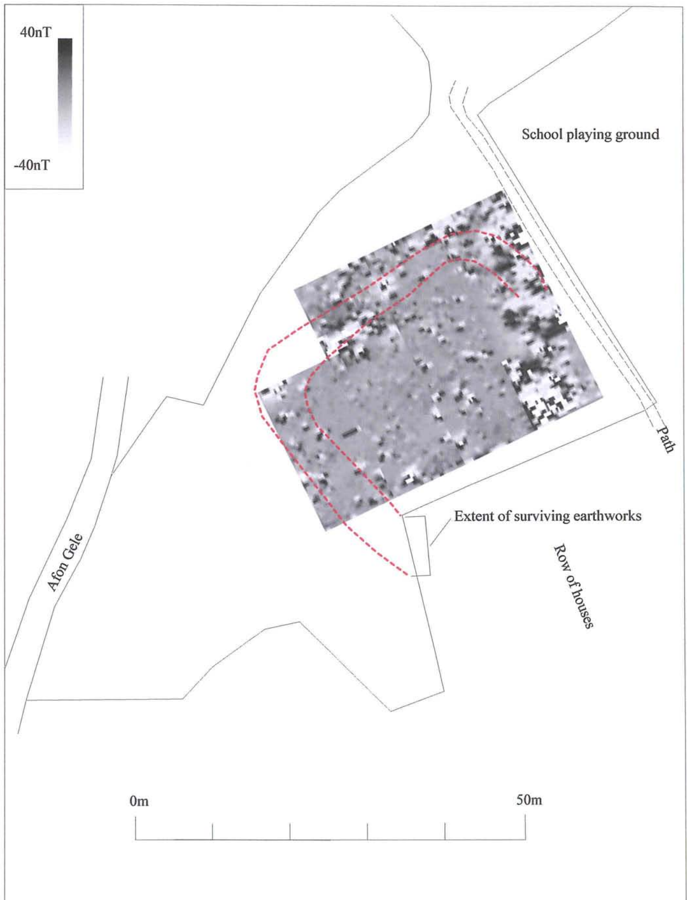
Fig. 2 Greyscale plot of the geophysics results showing the extent of the surviving earthworks
