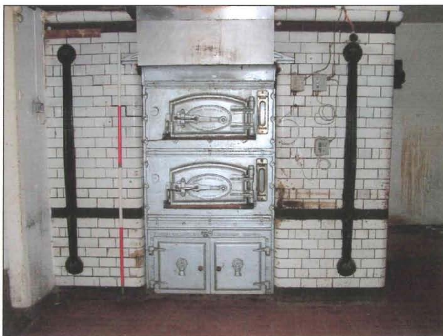
Plate 3 The oven, made by Thomas Collins & Co Ltd of Bristol (Photo CPAT 2575-062)
