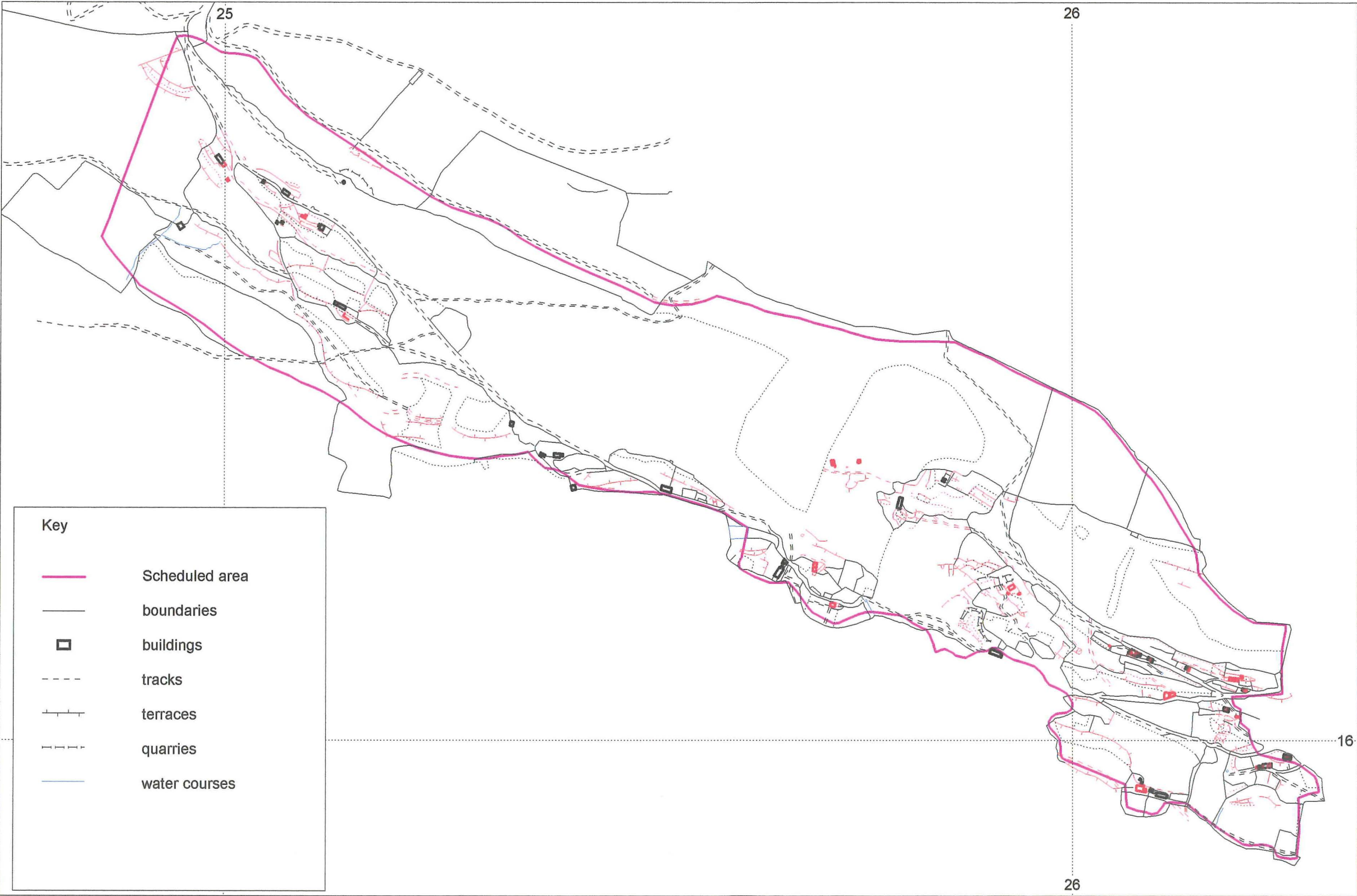
Fig. 5 Comparison between the digital mapping of Ordnance Survey 1st edition 1:2,500 map (black) and additional survey data (red), reproduced at 1:5,000
