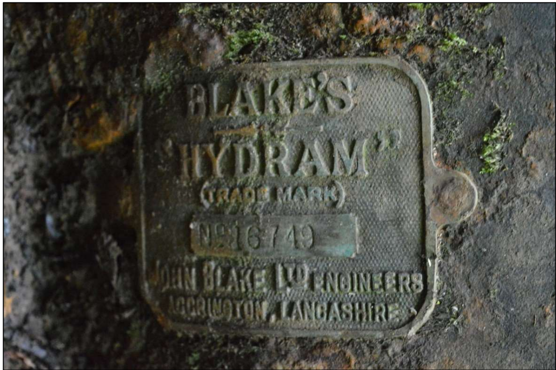
Fig. 10: Hydraulic Ram identification plate. CPAT 5007-0011
