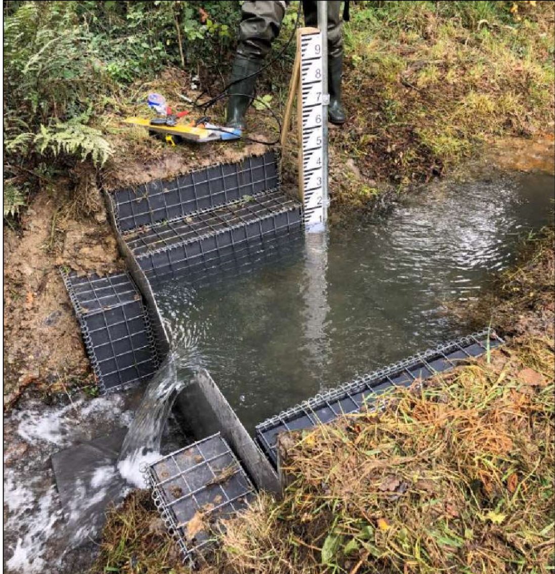
Fig. 15: An example of a typical temporary flow monitoring structure
